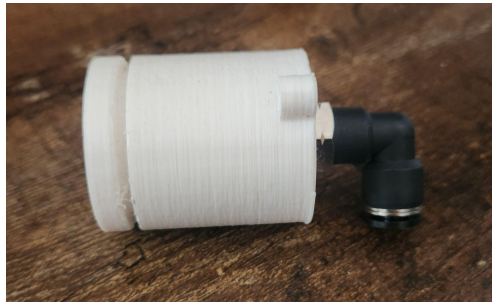
Figure 11: 3D Printed Pneumatic Adapter.
