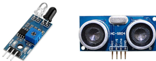
Figure 6: IR line detection sensor (left) and ultrasonic distance sensor (right).
