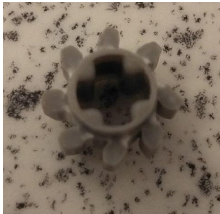
Figure 10: Catastrophic Gear Failure
